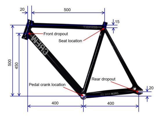
Figure. Bicycle frame structure (unit mm)
